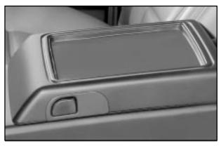
To open it, press the button on the side and swing the console lid open. The console includes CD holder slots and a tissue holder which is located on the inside of the console lid.
